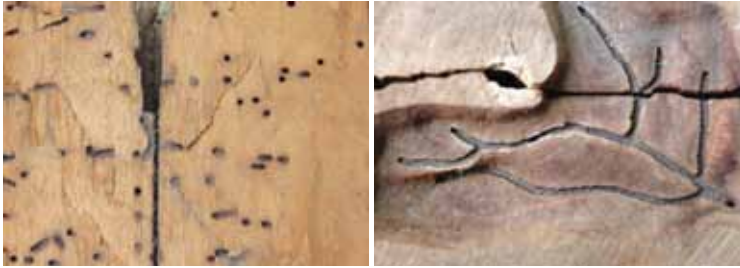
Figure 6.11. Attack by wetwood borer causes deep holes in wood
